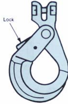
FIG. 7 SELF-LOCKING CLEVIS HOOK (CLOSED)
