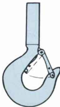
FIG. 13 SELF-CLOSING TIPLOCK LATCH (SHANK HOOK)
