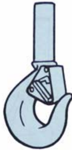
FIG. 10 SELF-CLOSING FLAPPER LATCH (SHANK HOOK)
