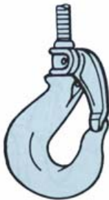
FIG. 9 SELF-CLOSING GATE LATCH (SHANK HOOK)
