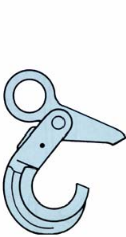
FIG. 6 SELF-LOCKING EYE HOOK (OPEN)
