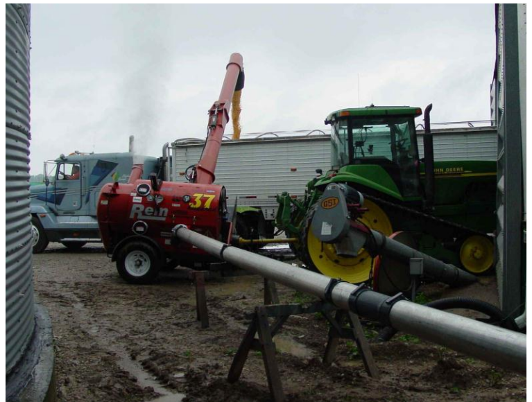
Exhibit 3. Stock photo of REM 3700 grain vac loading grain into truck ( image from www.rementerprises.inc.com )
