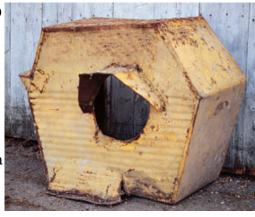
previously stated, evidence indicates that the youth was standing near the rotating flywheel clutch facing the farmer when his clothing was caught by the exposed clutch mechanism, most likely the spring-loaded drive-pin. He was killed instantly when he became entangled in the PTO.
