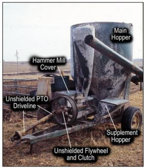
**#1:** ensure that PTO drivelines and other drive-line components are completely shielded to prevent worker contact with rotating machine parts.
