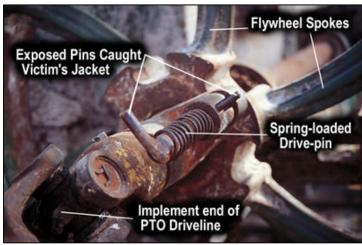
covering the flywheel, had been damaged and removed by the farmer 10 years prior to the incident.
