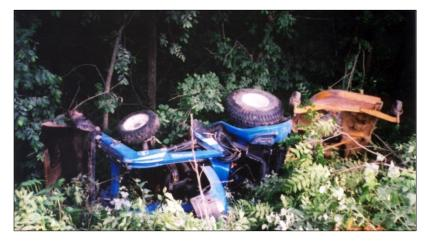
Scene involving a tractor overturn fatality where retractable ROPS was secured in folded-down position. *Photo courtesy of <u>Iowa FACE Program</u>*
