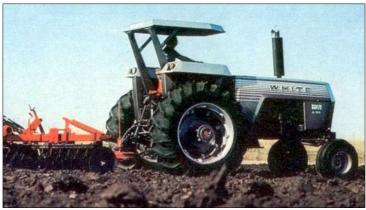
Tractor with 2-post ROPS. Photo credit: <u>www.TractorData.com</u>
