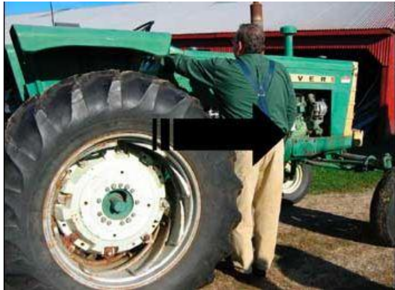
Depiction of an operator's hazardous position when starting tractor from the ground. Arrow shows movement of tractor left in forward gear when started.
