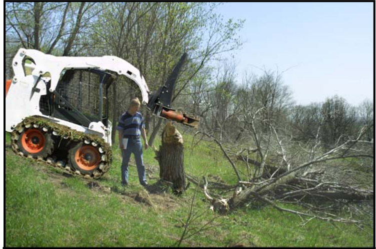
Electronic Image 1 - Approximate position of loader and raised tree shear attachment, looking from the side. (see note below)
