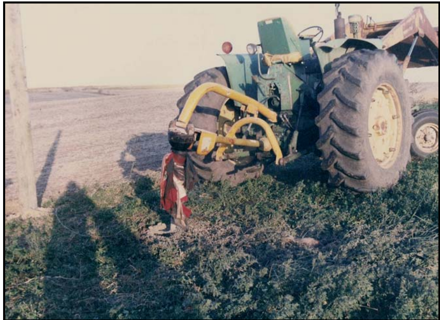
Photo 1 – Tractor shown with three-point hitch, PTO-powered posthole digger attachment as it was found early in the morning after the incident.
