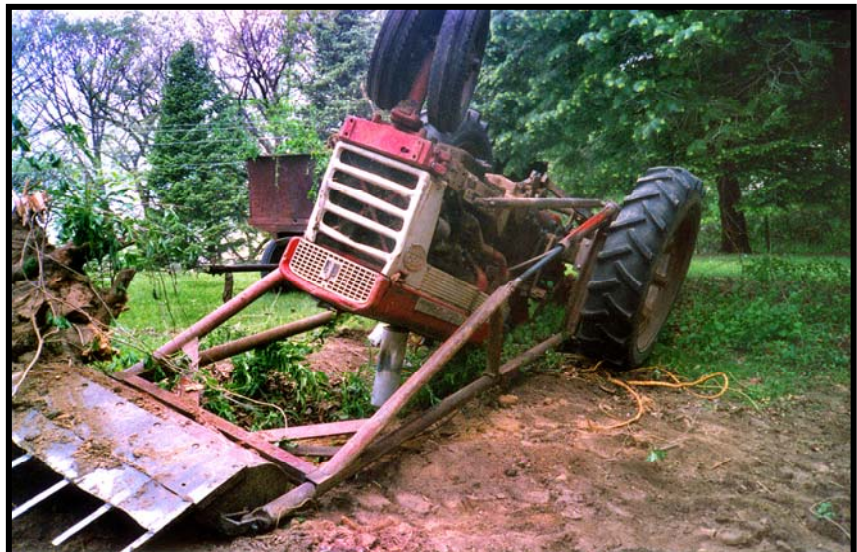
Photo 3 – Front view of the tractor, with the wagon uphill in the background, showing the front loader was raised prior to the overturn.
