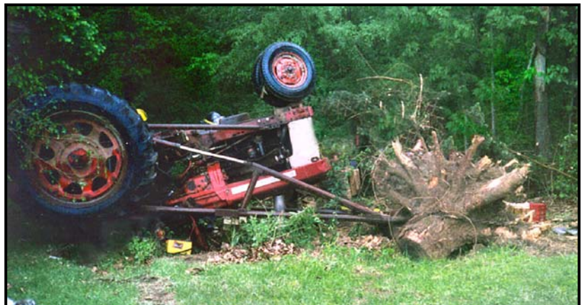
Photo 1 – Side view of the overturned tractor showing the raised front-end loader with the stump secured by a log chain.
